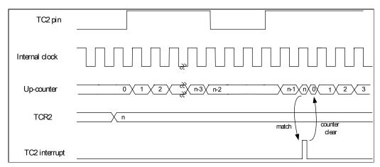
Fig. 5-21 Window Mode Timing Chart
